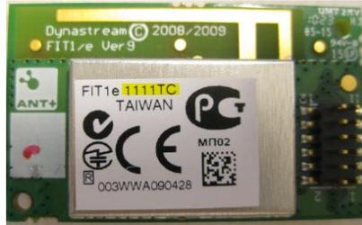
FIT1e modules version A and B produced **before April 2011** have different product stickers and often have some hand written marks on the PCB boards, as indicated in the picture below. Version A and B are not further identifiable through the product sticker.
