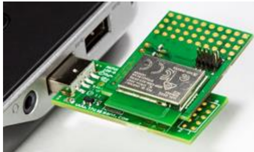
Figure 5-4. G.FIT Module Mounted on a USB Interface Board
